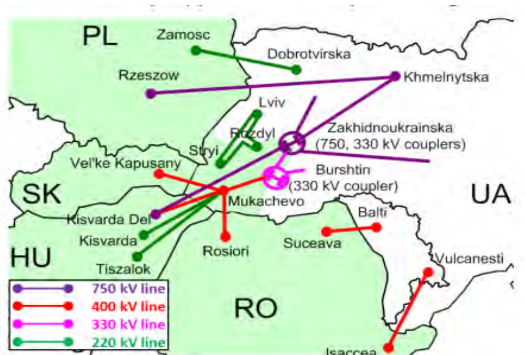
Figure 11 Schematic overview of the Ukrainian and Moldovan power system interconnectors with the surrounding ENTSO-E TSOs (The Rzeszow -Khmelnytsk NPP power line was rehabilitated to 400 kV) 3536
